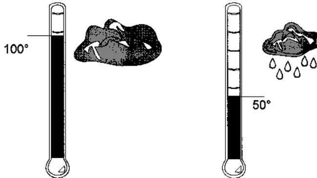
At a higher temperature the air holds more moisture      At a lower temperature the air holds less moisture
