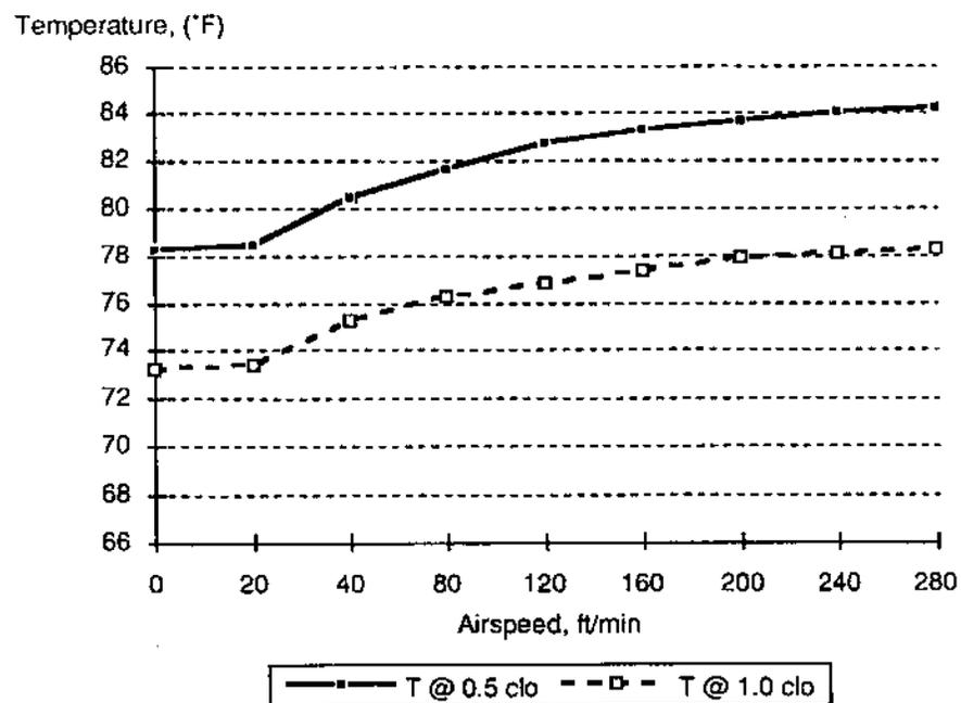
*Optimal comfort temperatures as a function of airspeed*
